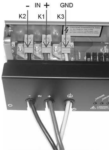
Figure 1. Cable connection for 24V and 48V inputs.
